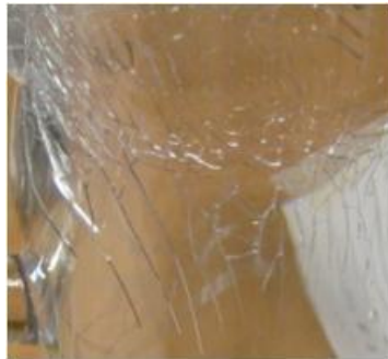
Un-annealed PC (severe cracks)
