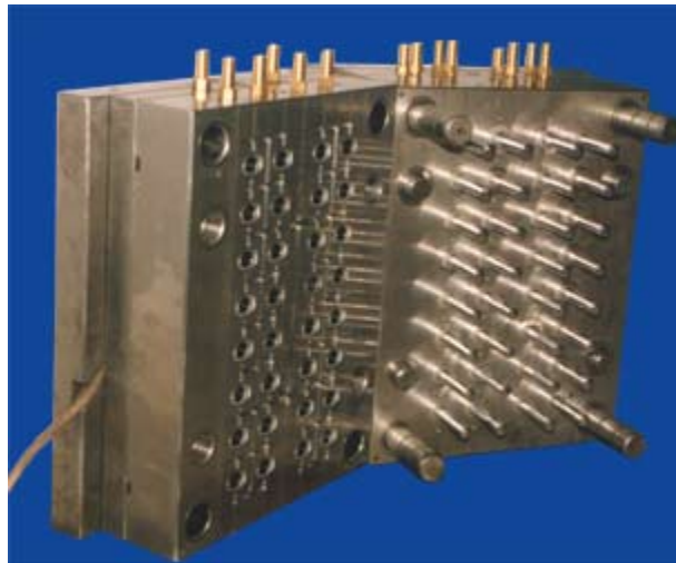
16 Cavity Mold for Surgical Blade Handles
