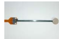
Gamma-radiated enzymatic-based glucose sensor (Cit Website, 2014)
