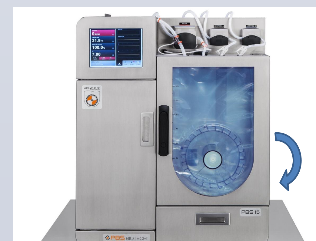
Figure 3: The Air-Wheel® system utilizes rising gas bubbles and converts them into rotational mixing power, lowering the amount of shear stress on the cells. Lowering the agitation of the system significantly reduces the amount of total air gassing. Photo courtesy of PBS Biotech.
